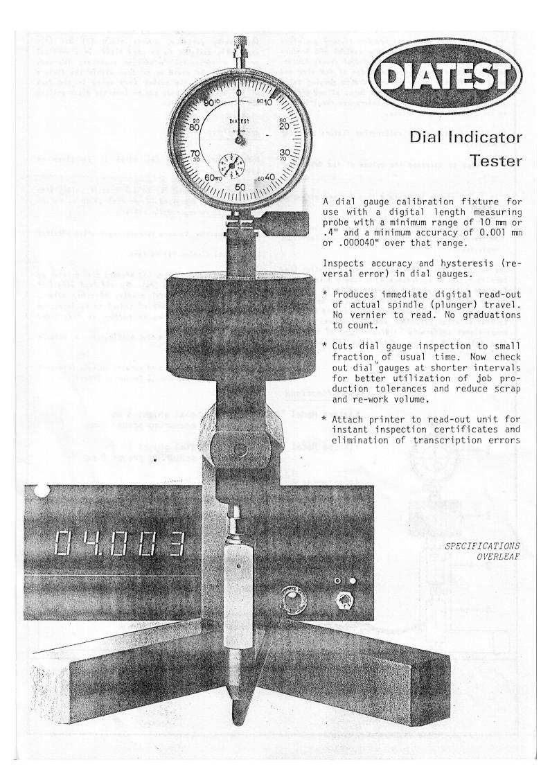
The DIATEST dial gauge calibration fixture satisfies an increasing demand by quality control and production engineers for ways to inspect dial gauges faster and in greater frequency. Knowledge of the size and position of dial gauge errors permits gauging tolerances to be narrowed which, in turn, allows greater utilization of job production tolerances resulting in an increase in "pass" volume.
